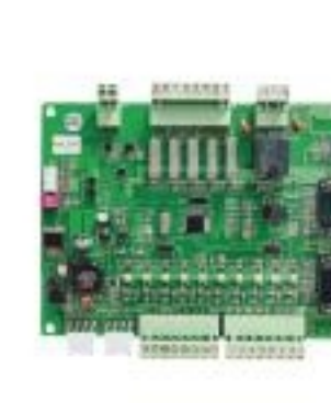
■ Car Top Control Board
